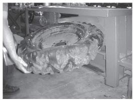
Place tire & wheel into the TC-300 crushing chamber. Place wheel with valve stem facing up. Center wheel over beam. NOTE: It is recommended that air be vented from tire.
