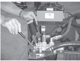
Operate Hydraulic valve handles. Pull valve handles towards operator to crush wheel. Push valve handles away from operator to return crushing wedge to starting position.
