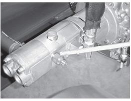
This adjustment controls low to high pressure shift point. If motor bogs down-loosen lock nut and turn Allen screw counter clockwise 1 / 2 turn and retry
