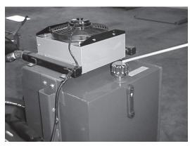
Check to be sure breather is installed in top of hydraulic reservoir.
