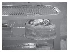
This photo illustrates the wheel being partially crushed.
