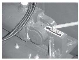
Periodically insert grease at the cylinder pivot.
