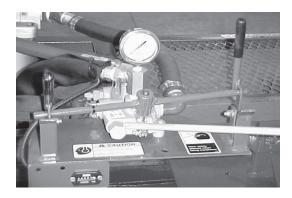
This photo illustrates the adjustment location of the hydraulic pump pressure to the valve. The gauge should read 2800-3000 PSI when the ram is fully extended. To increase pressure, first remove large Hex nut. Then using a Hex Allen wrenchturn adjustment screw to the right 1/4 turn at a time & recheck until pressure is 2800-3000 PSI.
