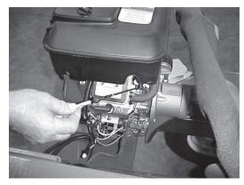
Check engine for oil and fuel levels. Turn on fuel valve, start engine using manufacturers operating instructions.
