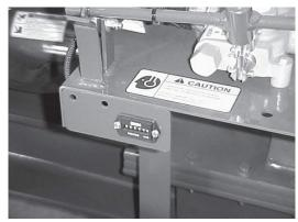
The Hour Meter indicates elapsed hours for proper engine maintenance service intervals.
