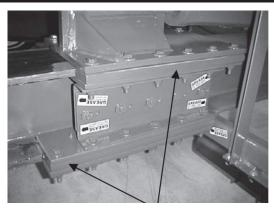
The crushing wedge has space wear bars on both the upper and lower slides. These wear bars may need adjusting. Loosen 6 upper and 6 lower cap screws and slide wear bars up to beam flange. Leave 1/32 clearance between beam and wear bar. If wear bars are worn too much, remove bars and turn side to side. This will give a new side to guide on. DO NOT ALLOW SLIDE BOLTS TO LOOSEN. KEEP BOLTS TIGHT TO 100 FT-LBS & ADJUST SLIDE PLATES IF NECESSARY.
