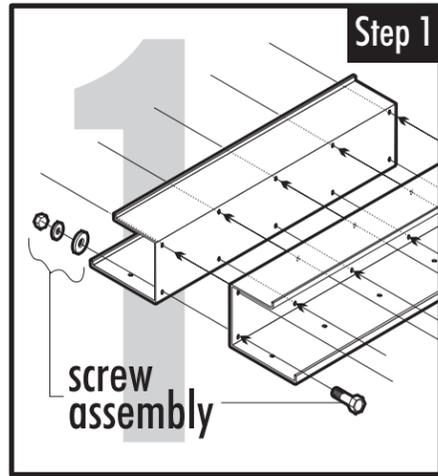
Attach the 2 TOP SHELVES (item # 11 on the left) together as shown using a total of 10 screw assemblies (item #'s 10,6,5 & 4)
