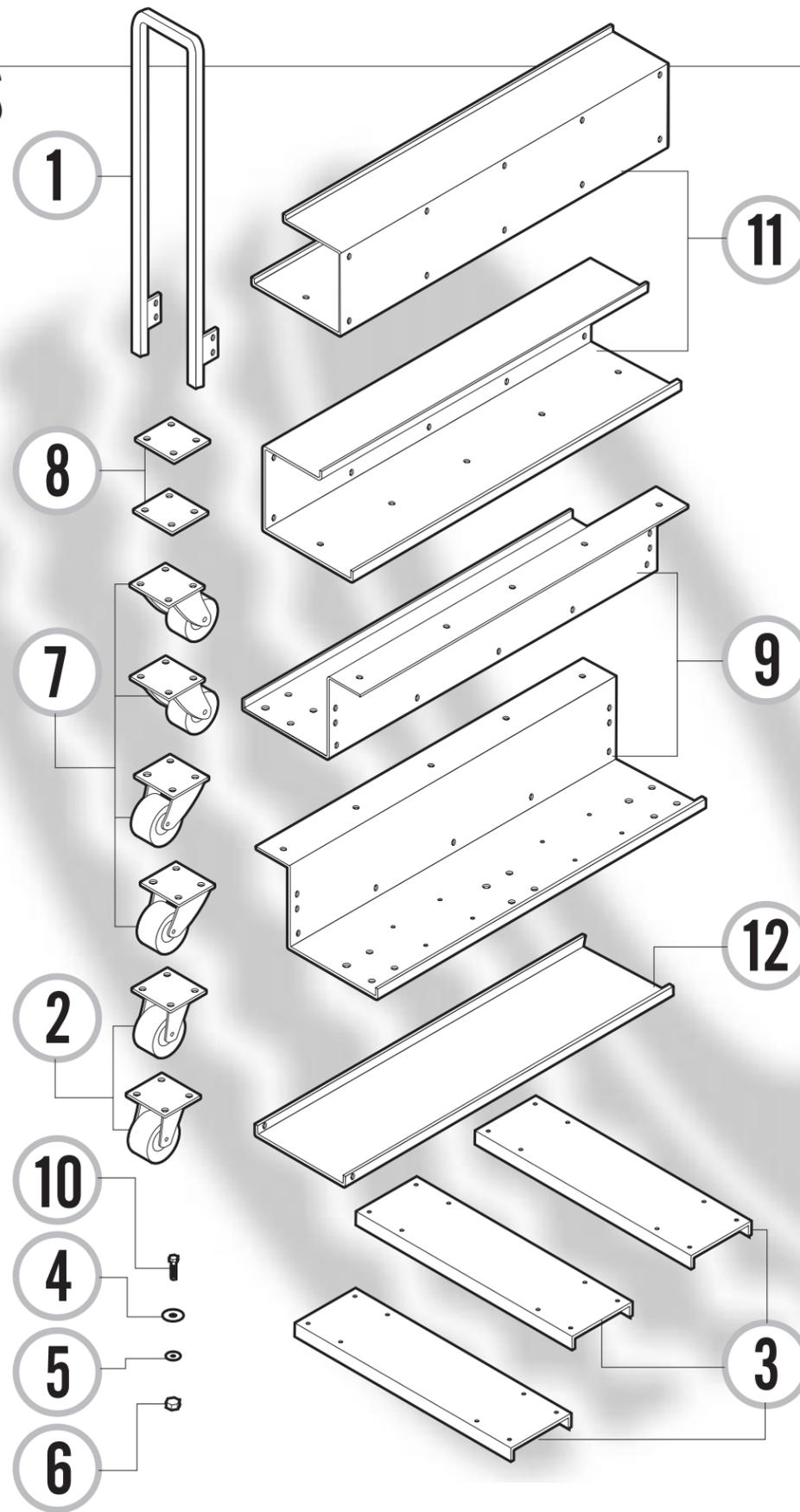
Attach the middle CHANNEL BRACE (item # 3) between the 2 MIDDLE CASTERS (item # 2), the 2 SPACER PLATES (item # 8) and the bottom of the BASE PLATES (item # 9). Thread 4 screw assemblies (per caster) through the 4 fore mentioned components
