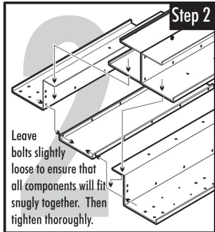
Attach the top lip of the 2 BASE PLATES (item # 9 on the left) to the previously attached # 11's, with 5 screw assemblies each. Attach item # 12 in the center of the 2 # 9's using 10 screw assemblies.
