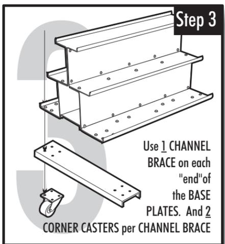
"Sandwich" 2 CHANNEL BRACES (item # 3) between the 4 CORNER CASTERS (item # 7) and the bottom of the BASE PLATES (item # 9). Thread 4 screw assemblies (per caster) through the 3 fore mentioned components
